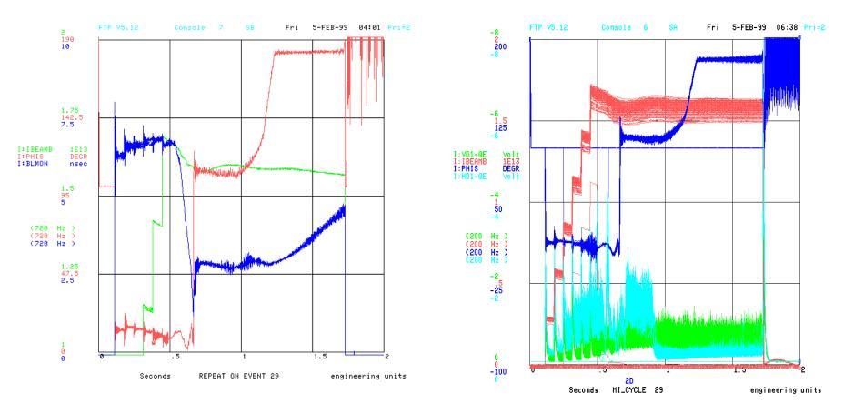
Max Intensity with no instability. ppp > 1.6e13 with >85% efficiency
