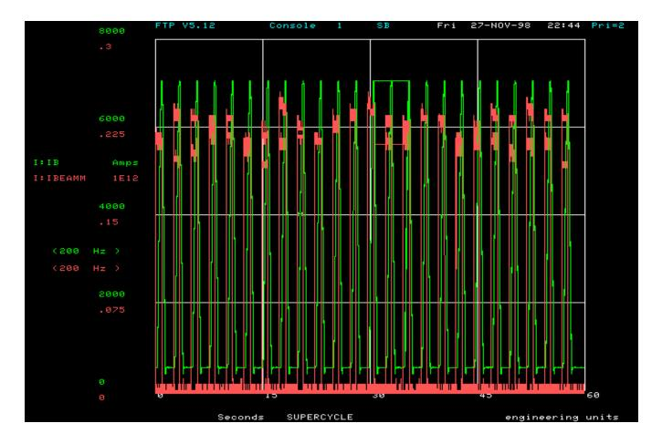
On Nov 28th 1998, We successfully ramped the Main Injector to 150 GeV with beam. The overall efficiency was ~85% at 150 GeV.
