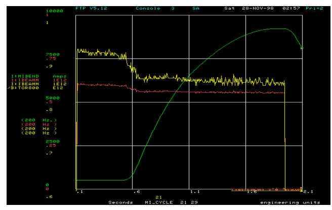
On Dec 24th 1998 Fermilab Main Injector achieved 2.2e12 protons/batch intensity @ 120 GeV. The overall efficiency achieved was ~75% at this intensity.
