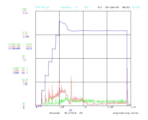
1-q error signals with the highest intensity observed so far. Even with the dampers off the error signals indicate no instability.
