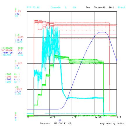
BLMON was increasing for 3-6 batch injection, with 5 turns from Booster. On Jan 6th 1999 Fermilab Main Injector achieved >1e13 protons/6 batch intensity @150 GeV. The Main Injector Commissioning goal was to achieve
