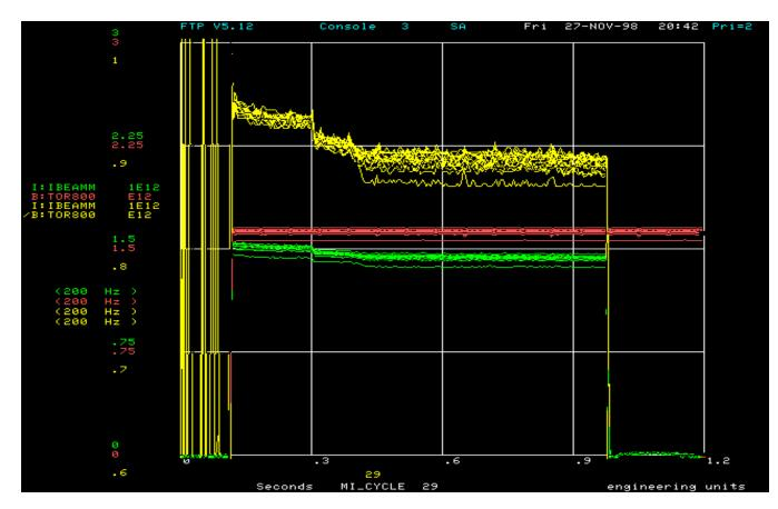
On Nov 27th 1998, We successfully ramped the Main Injector with beam at a repetition rate of 2.5 Sec. This satisfied the commissioning goal
